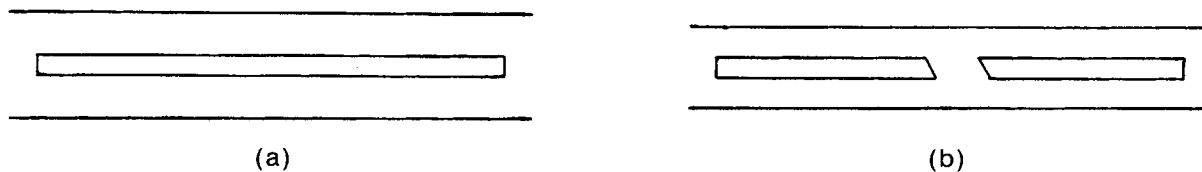
Figure 2 Schematic representation of an LCP microfibril embedded in a PP matrix fiber; (a) as-spun fiber and (b) drawn fiber.
